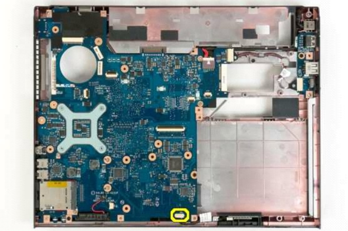
19. Disconnect the USB board data cable from the system board.
