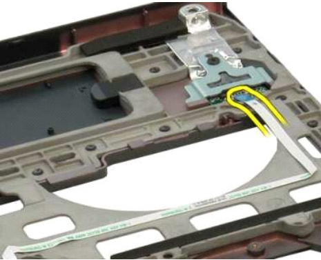
14. Remove the screw that secures the fingerprint reader bracket to the computer chassis.
